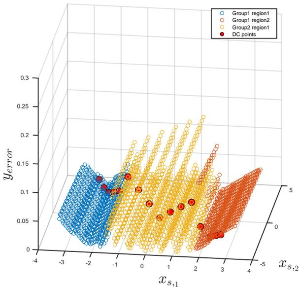
Fig. 9. Output deviation ( $y_{error}$ ) between the generated model, with three locations, versus the original netlist for the example form Section IV-A. The three used DC points for modeling exhibit the lowest errors.
