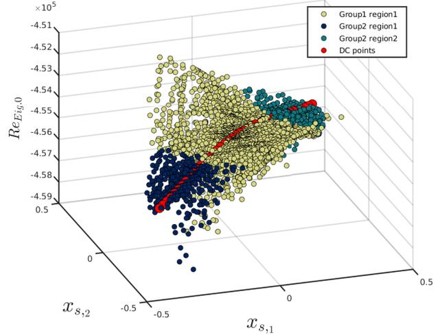
Fig. 7. Real part of the first eigenvalue plotted versus the shifted and transformed state space of the gm/C filter. The different locations of the HA are plotted in different colors. The DC operating points are plotted in red.
