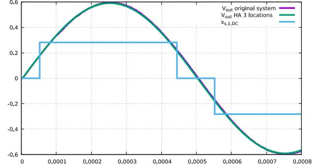
Fig. 8. Simulation results of the netlist versus the generated HA with 3 locations of the gm/C filter. The input of both systems is a sine signal with an amplitude and offset at 1.52V and a frequency at 1 KHz.
